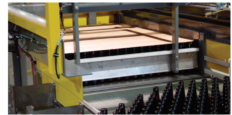
Optional front layer retainer bar to hold the front row of each layer for un-stable containers.
